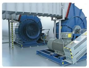
Unbalance is critical in fan installations (direct coupled or with belt pulley transmission)
